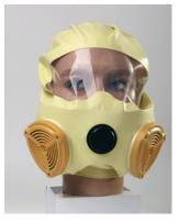
A personal respiratory protective device intended for self-rescue during emergency situations where smoke and hazardous fumes are present. The COGO provides users with short-term respiratory protection against smoke and Carbon Monoxide (CO) inhalation and filters the following gases: HCI, HCN and Propenal. The COGO mask complies with European Standard EN-403 and CE mark. The COGO has been custom crafted to meet the needs of the following industries:
