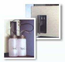
• Conveniently located peristaltic pump, syringe, water and waste bottles (with level sensors) for easy accessibility and maintenance.
